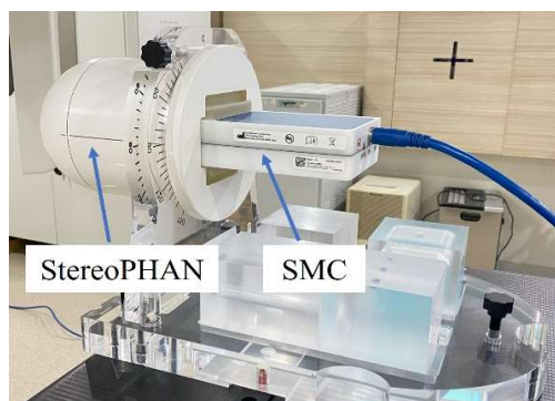
Figure 1. SRS MapCHECK (SMC) in StereoPHAN phantom.
